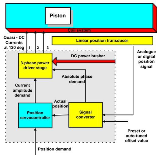
**In its application to motion bases and stabilised platforms** the electromagnetic ram technology provides:-
