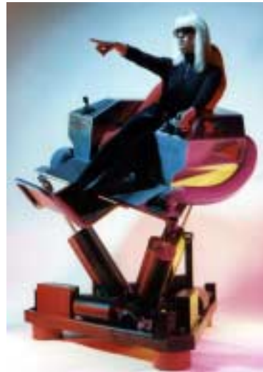
3-axis base showing power drivers
