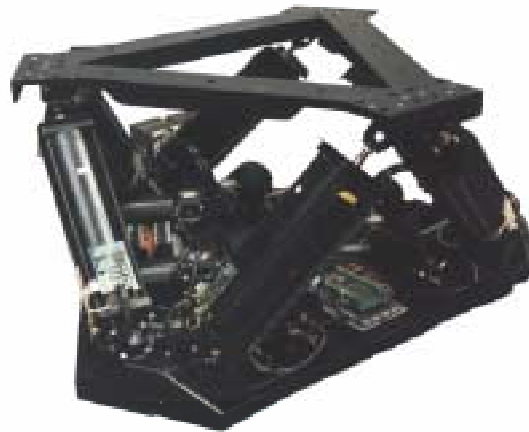
Commutated ram 6 DOF motion base
