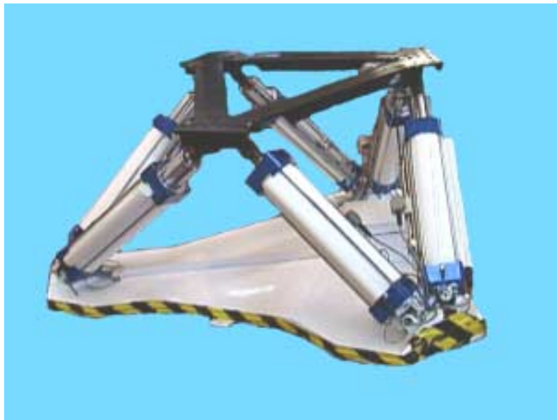
Advanced Motion Technologies 6 DOF Motion Base
