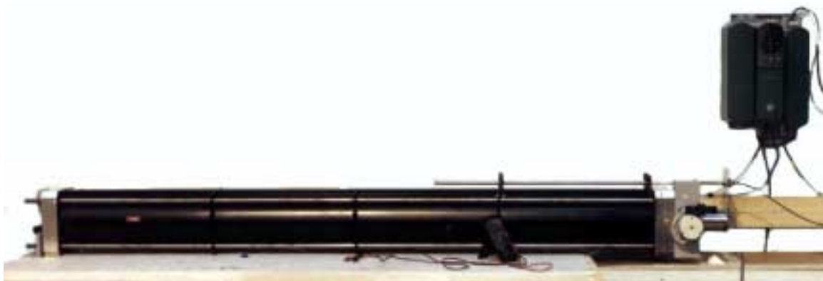
Assembly Industries 5 KN thrust, 1.5m stroke ServoRam on bench test
