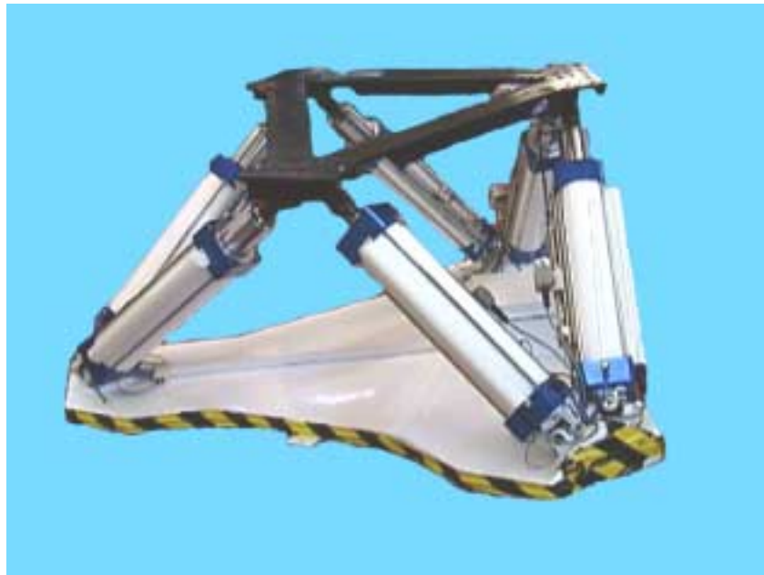
Motion base for a professional training simulator, using industrial ServoRams™
