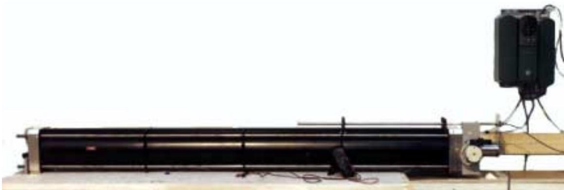
**Assembly Industries 5 KN thrust, 1.5m stroke ServoRam on bench test**
